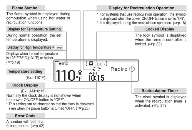
Note: As shipped from the factory, the remote controller is set to display in °F and gallons. To adjust the display to °C and liters, refer to the Installation Manual.
