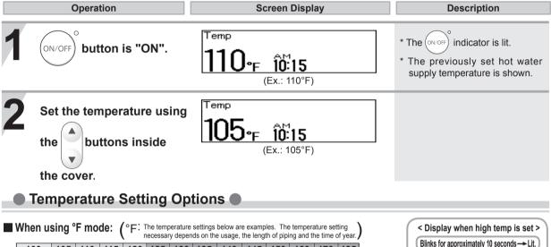
105 | 110 | 115 | 120 | 125 | 130 | 135 | 140 | 145 | 150 | 160 | 170 | 185 Washing Shower, hot water supply, etc. High temperature \*Initial factory setting is 110°F
